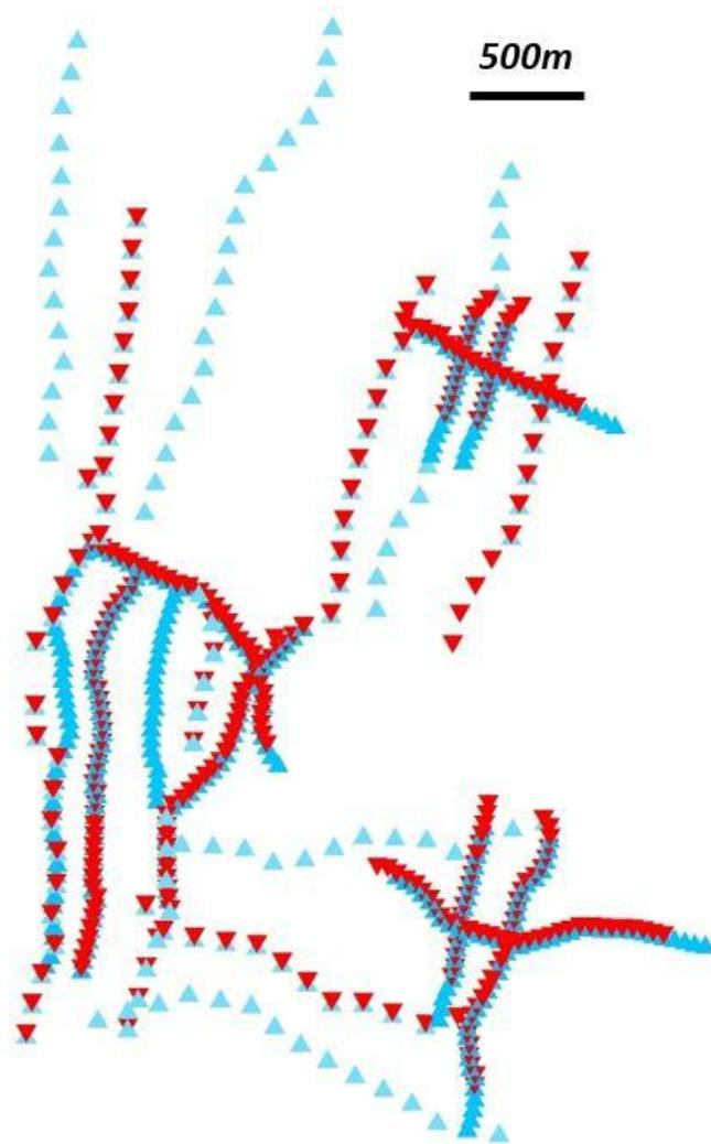
Figure 3. Plan view of customised irregular trilinear 3DIP array layout with electrode locations (blue = Rx, red = Tx).
