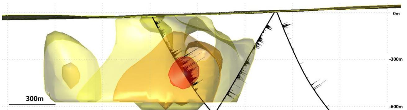
Figure 4. Cross-section of higher modelled 3D chargeability shells (yellow = weak, orange = moderate, red = high) with sulphur content in drilling (black traces).
