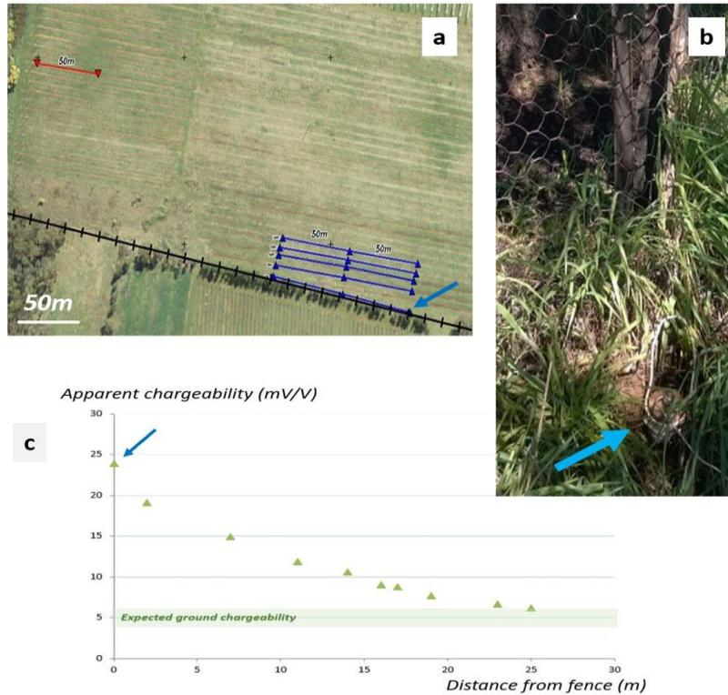
Figure 1. IP surveying results near a grounded metallic fence. (a) Location of survey electrodes (blue = Rx, red = Tx) and fence (in black) over aerial photography. (b) Photography of Rx electrode next to the fence. (c) Measured apparent chargeability values plotted against orthogonal distance from the fence. The blue arrow identifies the closest reading from the fence.
